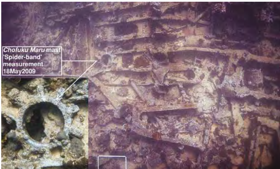
Figure 185. Mast spider band measured on the Chofuku Maru wreck site in 2009 (Kalle Kasi and Patrick Baker).
