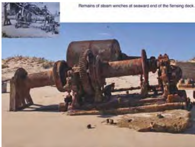
Figure 20. Remains of steam winches at seaward end of flensing deck (Colin Cockram).
