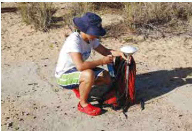
Figure 24. Corioli Souter setting up the OmniStar and DGPS (Myra Stanbury).
