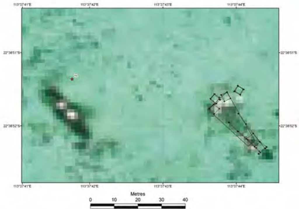
Figure 71. Plan of the Fraser Island Lighthouse and the Fin wreck site drawn from Photomodeler and superimposed on a GIS with aerial photograph (Jeremy Green).
