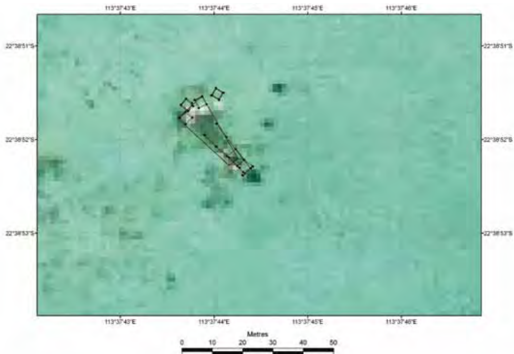
Figure 70. Plan of the Fraser Island Lighthouse drawn from Photomodeler and superimposed on a Geographical Information System (GIS) with aerial photograph (Jeremy Green).
