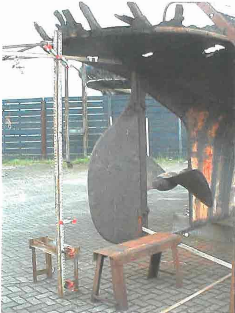
Figure 5. Scaffolding for taking lines (Joel Gilman).
