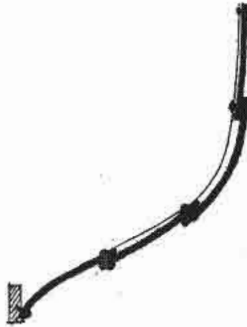
Figure 3. Strake overlap detail (Don Alexander).
