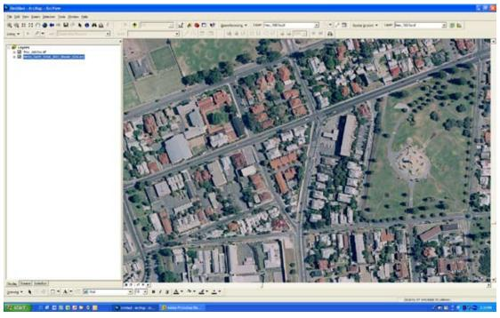
From now on in all further applications of Control Points the two images will be approximately on top of each other so all you will have to do switch the top layer on and off to see MOSAIC lying below. The image below shows the Georeferencing after inserting the second control point. Notice that the coastline at the bottom does not exactly match up, because we have only used two control points.
