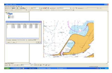
Click on Rectify in Georeferencing drop down and save rectified map. Delete original and replace with Rectified map RectifyNMoleAdm.tif in layer.
