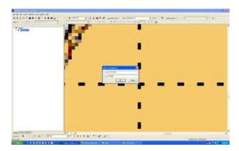
On clicking OK the image will disappear (because it has moved in geographical space) and you will have to use Zoom to Layer to relocate the image. Repeat for the three other points. You can check the points in the Link Table to ensure everything is correct.
