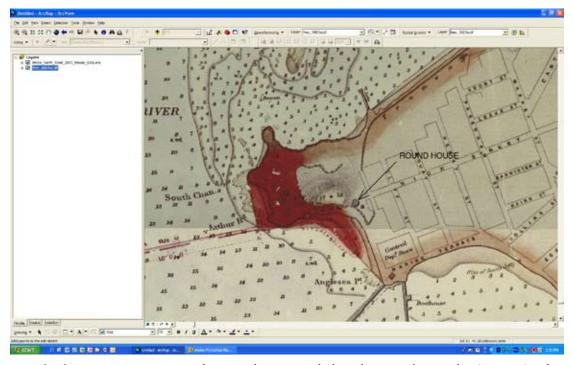
Go back to MOSAIC zoom to the Round House and place the second control point. Notice there will be line following the cursor with the control point tool. This line is joined to the first control point on FREO. If you do some other action between clicking on the first Control Point, so that the Add Control Point Button become deactivated, simply click on Control Point button and the tool will become active again.
