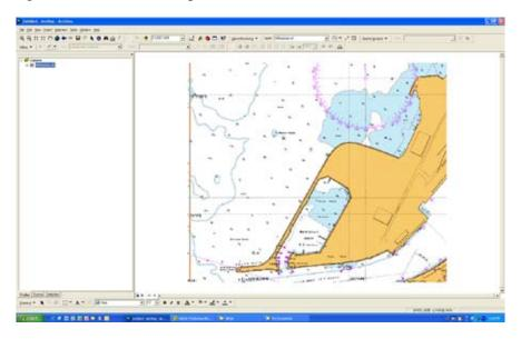
Activate the Georeferencing Tool Bar, select Layer and select Add Control Point. Zoom to the intersection of 115° 44'E and 32° 03'S. Click on intersection and then Right Click. This will give you an option box with Input X and Y or Cancel Point. Select former. Enter values as shown below.
