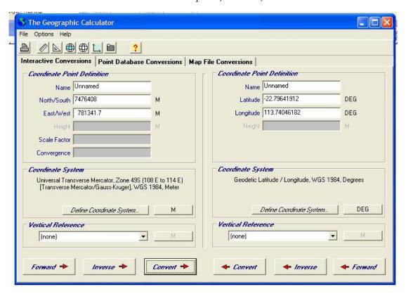
On the left hand side is one set of coordinates (usually the Input coordinates) and on the right hand side is the output. In the Coordinate System box choose Universal Transverse Mercator for the Group, enter the correct UTM Zone in System drop down. Select GD94 for the Datum and Metres for the Linear Unit (see below).
