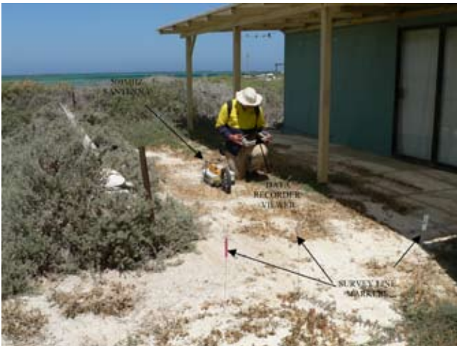
Figure 28. GPR acquisition system used on Beacon Island (Photo: Tristan Campbell, Geoforce).
