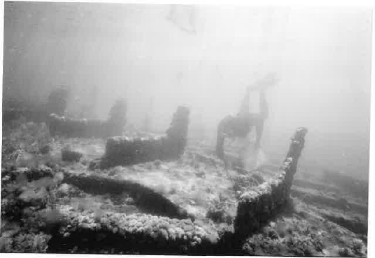
69) Upper deck beam knees on collapsed hull plating. Crown of England.
