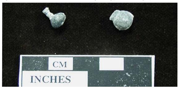
Figure 14. Samples from UNID 4604, showing evidence of sprues (Photo: Jen Rodrigues).
