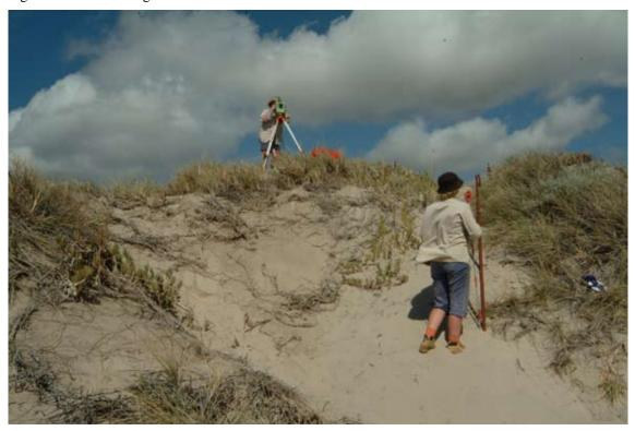
Figure 29. Surveying with the Total Station.
