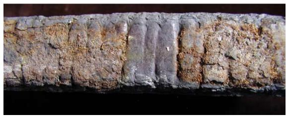
Figure 15. Striations along the edge of the lead fitting (UNID 4605) (Photo: Jen Rodrigues).
