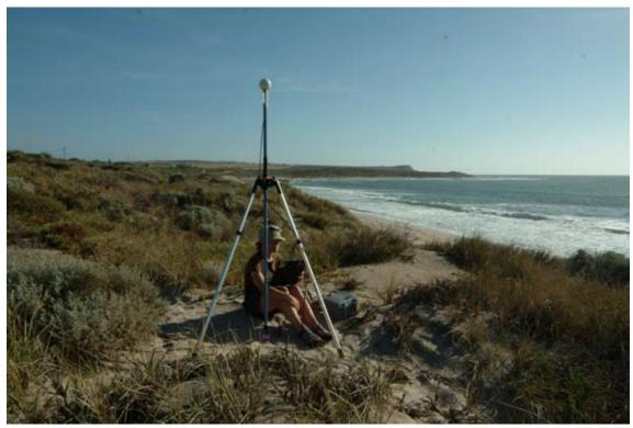
Figure 28. Recording with the DGPS.
