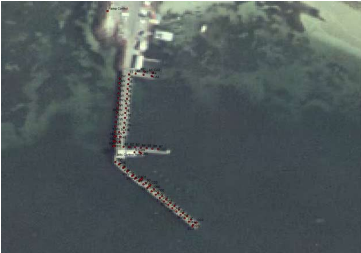
Figure 2. Total station survey of the existing Town Jetty piles.
