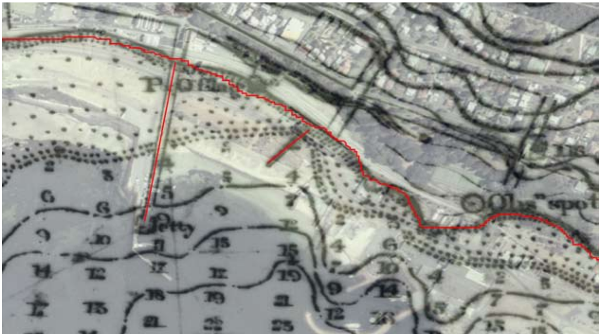
Figure 23. Trace of the original shore line taken from a semi-transparent georeferenced 1873 chart and superimposed over a contemporary aerial photograph.
