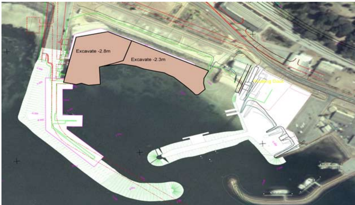
Figure 10. Plan showing the proposed development and the proposed dredged area in white (upper left).
